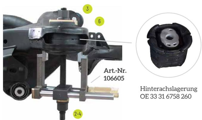
AUSBAU HINTERACHSBUCHSE HINTEN
