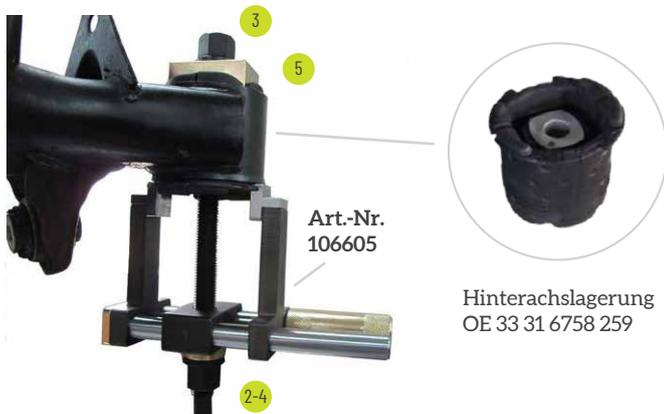
AUSBAU HINTERACHSBUCHSE VORNE
