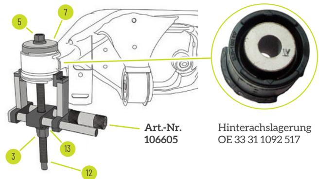
AUSBAU HINTERACHSBUCHSE HINTEN
