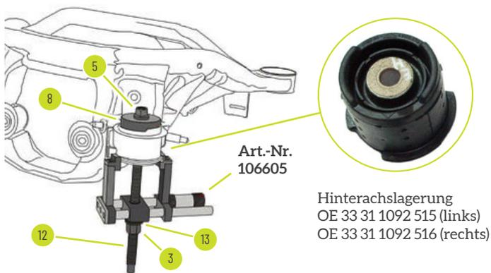
AUSBAU HINTERACHSBUCHSE VORNE
